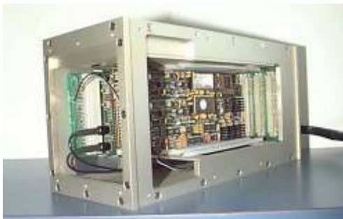
Figure 201. Typical ARC controller
