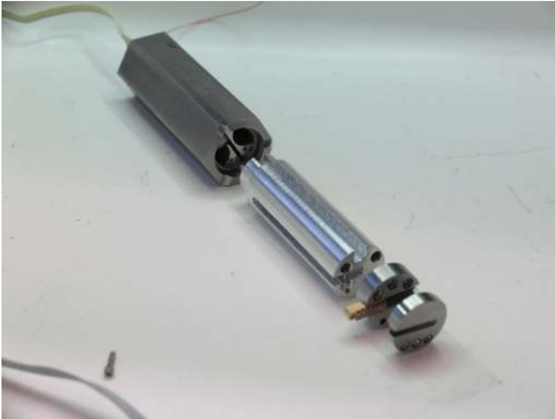
Figure 105. Disassembled LBNL actuator of the 1.92 cm hex size. The SIDE/GTC actuator would be somewhat larger, with a 2.92 cm hex size.
