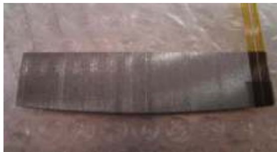
Figure 122: The pseudo-slit output of the IFU bundles of VIRUS. The fibers are arrayed on a precision grooved plate that sets the spacing and angle between fibers. The fibers are arrayed perpendicular to the back surface of a cylindrical lens bonded to the convex surface of the plate. From de Hill et al 2006.
