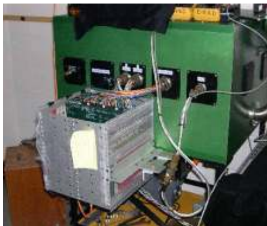
Figure 203. A Monsoon controller.
