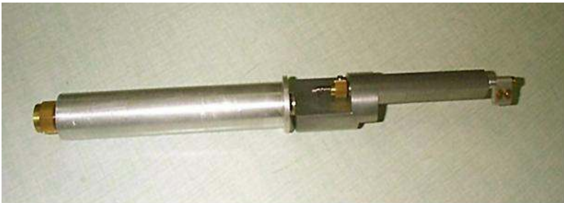
Figure 108. LAMOST fiber actuator on the bench for testing at Lawrence Berkeley Lab. The concept is very similar to the LBNL fiber actuator.
